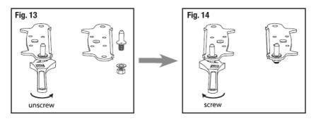
5. Refit the bracket fitting the bottom hinge pin. Replace both adjustable feet (Fig. 15). Transfer the lower door to the proper position.
