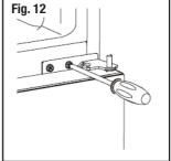
Carefully lay down the refrigerator and remove the levelling legs, then unscrew the lower hinge using a Phillips head screwdriver (Fig. 13).
