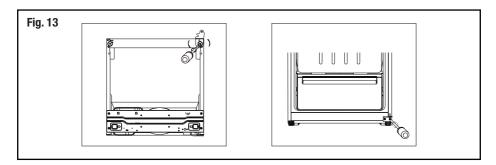
Unscrew and remove the bottom hinge pin, turn the bracket over and replace it (Fig. 14).
