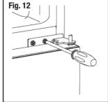
3. Carefully lay down the refrigerator and remove the levelling legs, then unscrew the lower hinge using a Phillips head screwdriver (Fig. 13).
