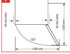
consumption and running costs. Allow at least 10 cm clear space at the back and 5 cm at the sides (Fig. 1) so air can circulate freely around the fridge.
